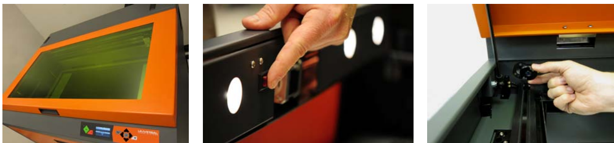
Figures 7, 8, 9: Changes to PLS6MW, from left: Safety Glass, Lights, Magnetic Collimator
